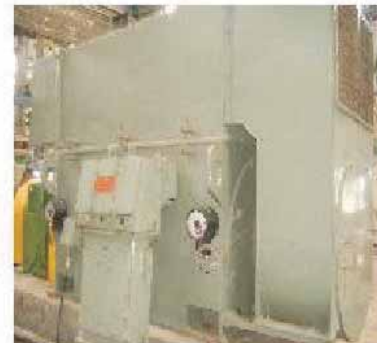
Stoppage of NBKP Soft wood Refiner moto in pm2 by optimising the processe like reducing the soft wood from 20% to 12%.
