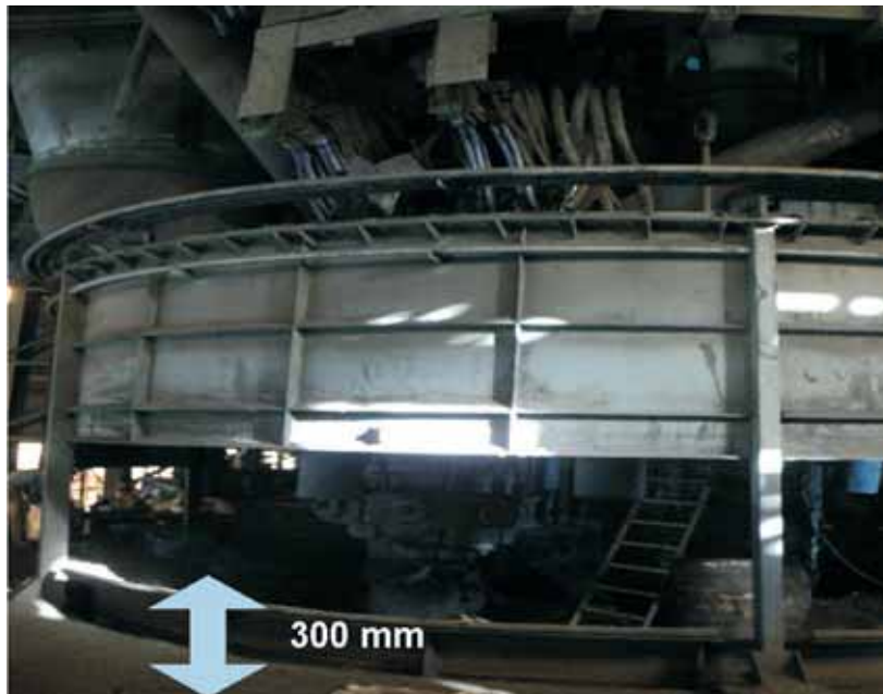
Raising of SAF Shell height by 300 mm shown by arrow
