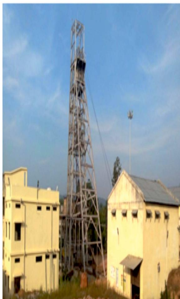
Excavation of manganese ore about 110 meters below ground is being carried out by cut and fill method, an inclined approached to underground from surface is used for transportation of ore from underground by using an electrical hoist, As the deposit of manganese are proved below ground in some other sections, a new vertical shaft 1sinking project is in progress after implementation of new system production capacity of mine will be increased.
