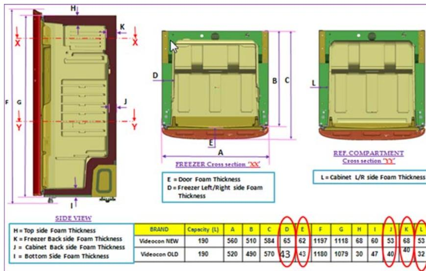
Figure showing increase in Foam thickness done and table below shows the difference in the foam thickness in old and new design.
