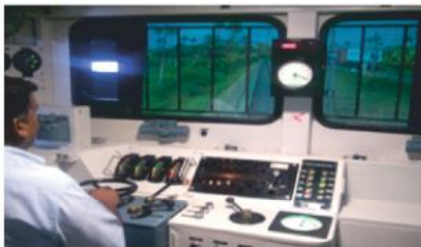
Intensive use of Loco Simulator for training of Loco Pilots and their monitoring by downloading energy data
